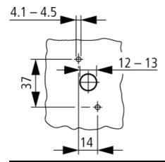
Diameter of drilled hole Door
