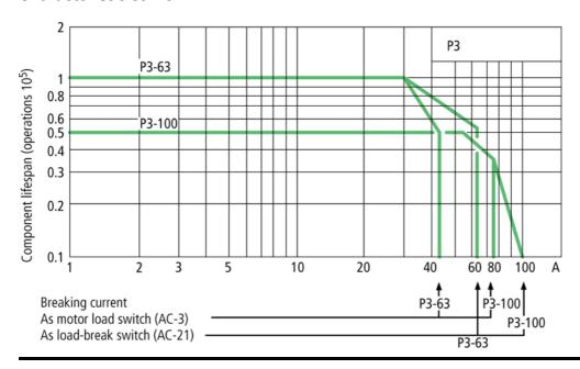
For utilisation category AC-4 (extreme load: 100 % inching, reversing or plugging) The blocked rotor current of the motor should not exceed the rated current of the switch for AC-21A to ensure a reasonable device lifespan.
